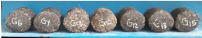
Fig. 8. Deformation of specimens after Marshall testing at flow of 12 mm.
